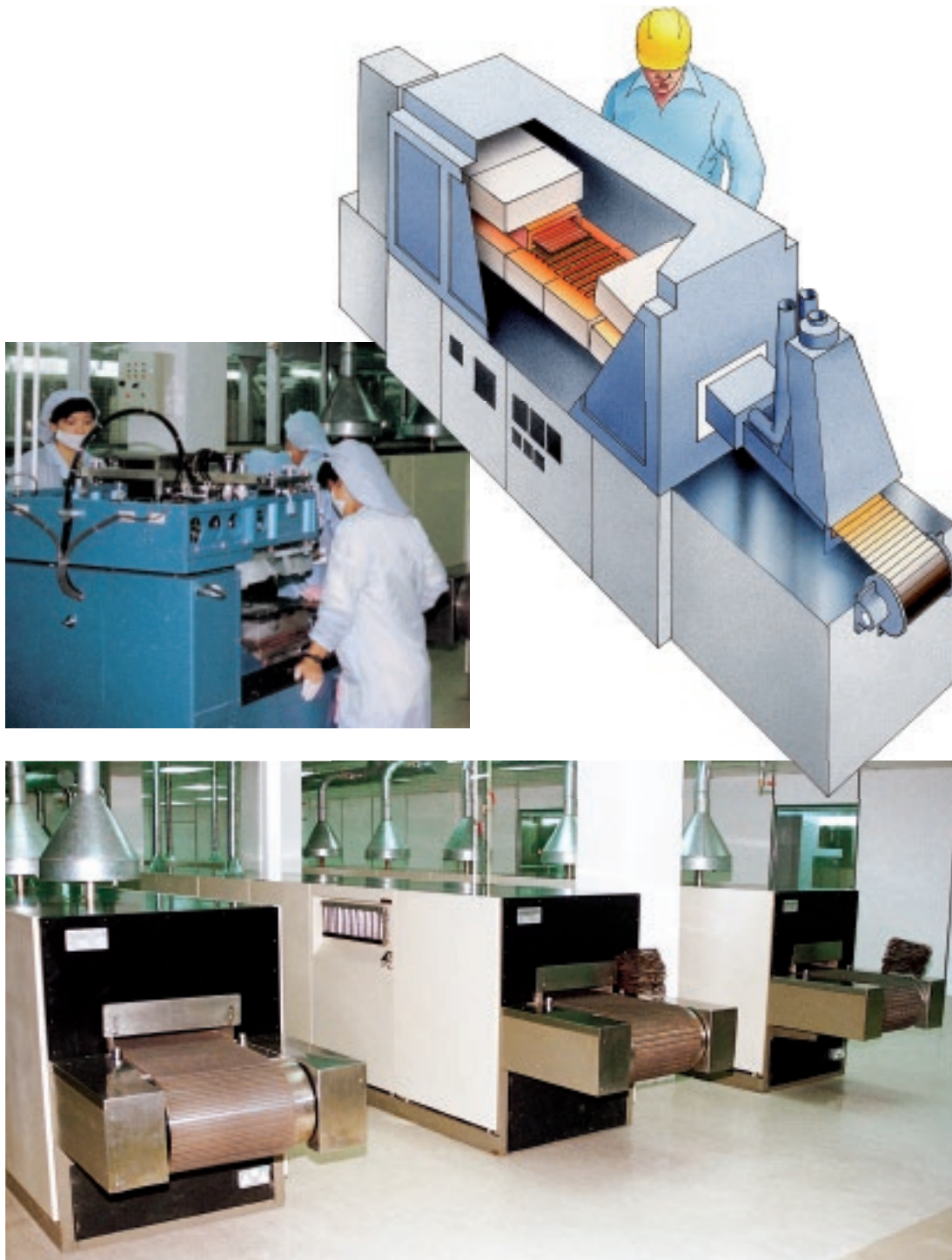
Fig. 25 Fibrothal modules used in a conveyor belt furnace.
