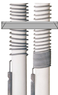
Comparison between Kanthal APM (left) and conventional FeCrAl (right) after 1250 h at max 1225°C element temperature.
