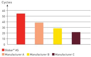
Cyclic test: Globar<sup>®</sup> AS vs. other manufacturers' elements. 100 hour cycles at 1425°C (2600°F).
