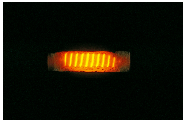
Glowing coil inside tubular heating elements.
