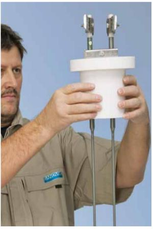
6. When determining the position of the element holder, it is of the utmost importance to ensure that the tapered transition between terminal and heating zone comes fully below the hot face of the furnace lining. If not, there is a risk that the part of the heating zone which is inside the lining may become overheated. When connecting the installed elements, the aluminum braids should first be bolted to the elements and then to the busbars.
