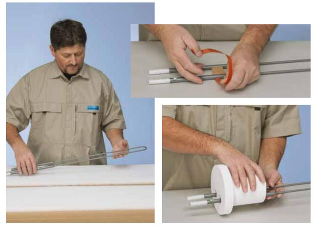
2. When unpacking, care should be taken to avoid any bending or twisting.
